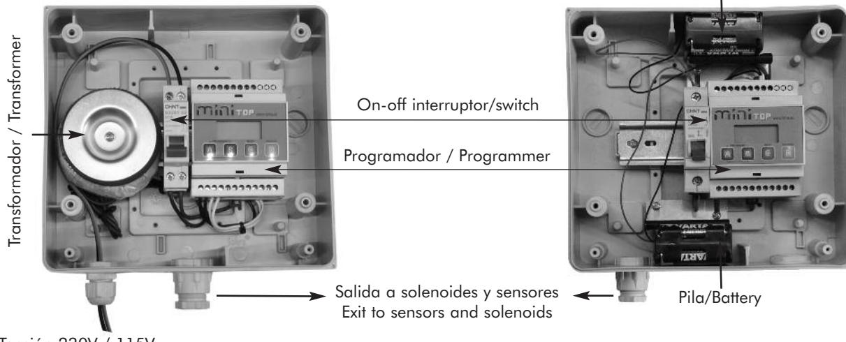
**Esquemas de conexión / Connections Schemes / Schémas de connexions**
